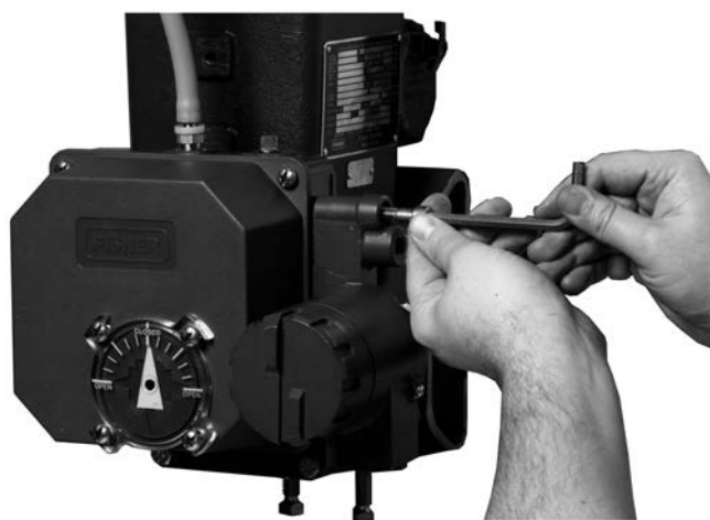
Figure 24. Removing the Converter Mounting Screws
