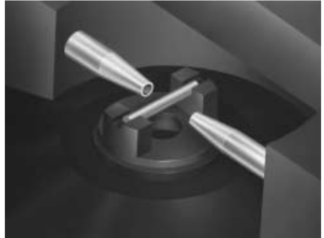
Figure 2. Detail of Deflector/Nozzle Pilot Stage
